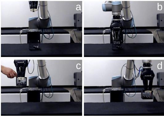
Fig. 10: Movement adaptation experiment. The robot generates the required movement trajectories in its end-effector and finger position spaces, automatically perceiving the task-related features such as the weight and shape of the object through its sensors (proprioception and force/torque readings). <https://youtu.be/cPKOIaf0mUc>
