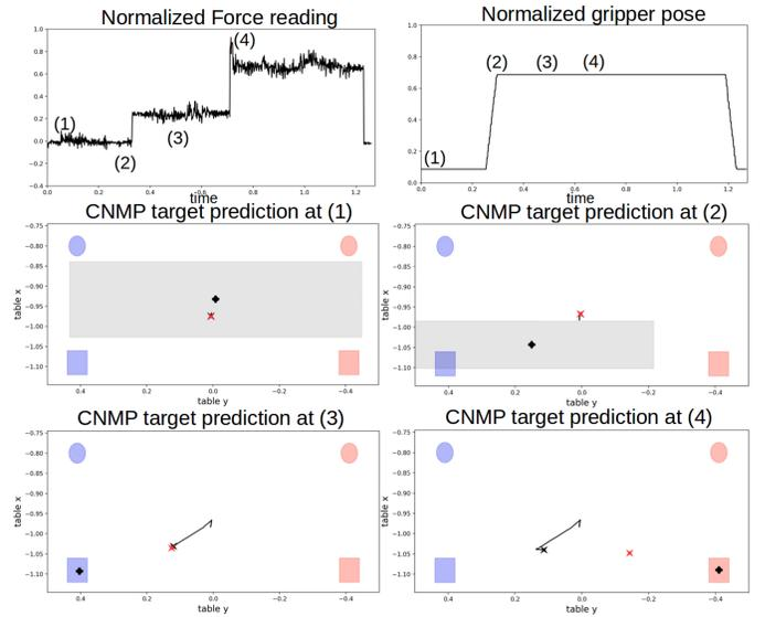
Fig. 11: Online conditioning and adaptation to unexpected changes during motion execution. Final position estimations are shown at 4 timestamps with black dot and gray shade. Container is approached (1), grasped but not lifted (2), lifted and carried (3), made heavier (4).
