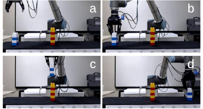
Fig. 7: Experimental setup and snapshots from demonstrations in the obstacle avoidance task where heights were provided as parameters.
