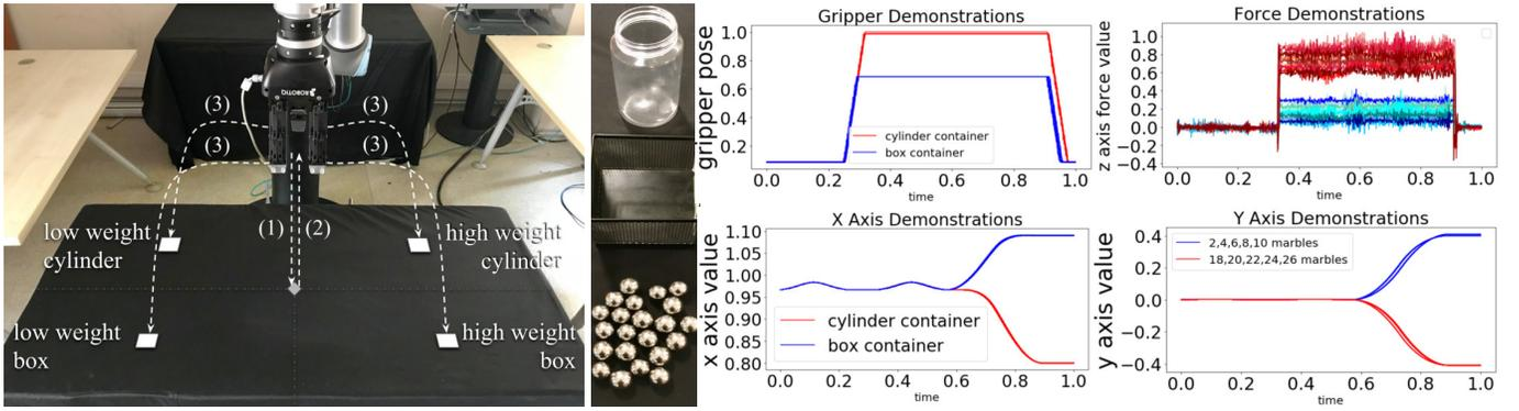
Fig. 9: The experimental setup for pick-and-place task where the placement position depends on the weight and shape of the container. On the left, the movement trajectories for different configurations are provided: The container is reached and picked-up (1), lifted (2), and carried toward target position (3). On the right: demonstration  $SM$  data.
